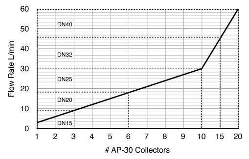
b) Maximum total flow-rate through any collector is 15L/min / 4gpm (~1m/s)
