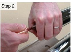
Holding spring plate in place, pull out each heat pipe by >150mm. (This allows easy insertion of the heat pipe into the header port.)
