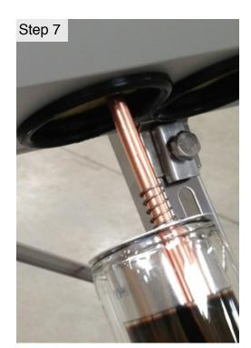
Lubricate outside of ET with water. (DO NOT spray water inside ET.)
