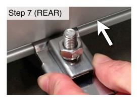
Push rear attachment plates tight into rear groove and tighten fully then tighten front attachment plates.
