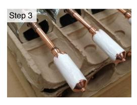
Coat each heat pipe with THIN layer of heat transfer paste.
